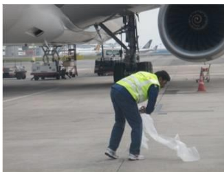
Removal of FOD
