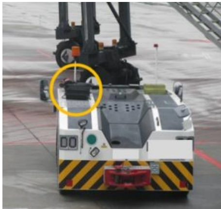
Example of wheel chock left unsecured on airtug
