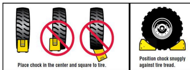
Sample of proper wheel chock placement
